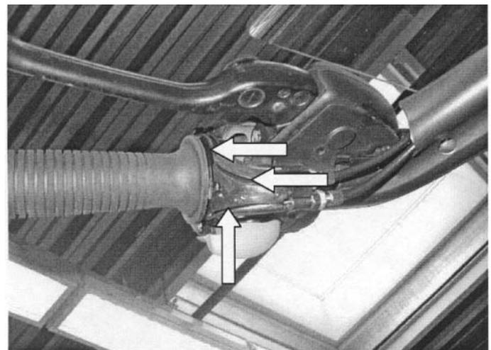
Spray the exposed parts of the throttle cables (**arrows**) with the dry lubricant mentioned above.
