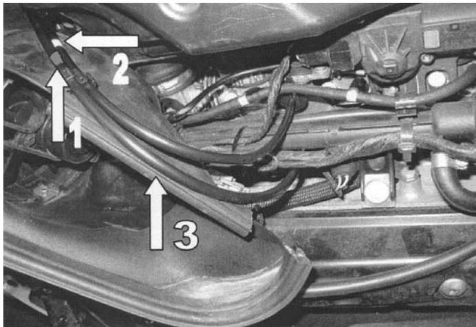
The throttle cables then have to be routed between the air filter box and the fan cowl, passed underneath the coolant hose and along the fairing bracket.
