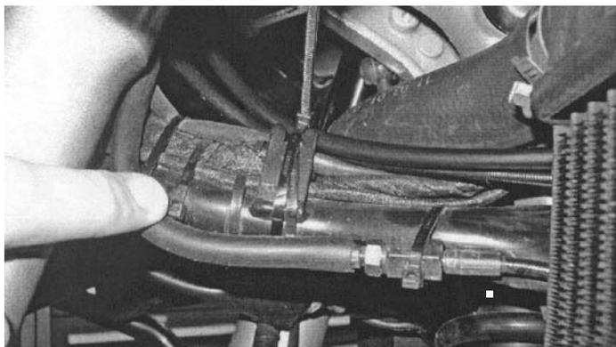
Route the throttle cables through the largest possible radius between the traverse of the fairing bracket (**Arrow**) and the threaded fastener (**Star**).
