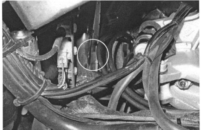
From the point of exit (**Circle**), the throttle cables have to be routed as shown. The arrow shows how they are secured with cable ties.. Here again it is important to ensure that the cable ties are left loose.
