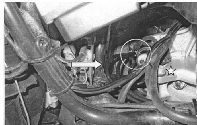
The circle indicates the safe margin of clearance between the throttle cables and the fairing bracket.
