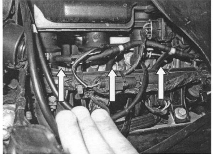
Once the throttle cables have been adjusted, it is important to check that the micro switch (**arrow**) of the cruise control system trips correctly. With the handlebars turned all the way to the left and right, the switch must trip with an audible click when the throttle twistgrip is turned slightly (approximately 10° according to the Repair Manual) in the forward direction of travel. Follow the instructions in the Repair Manual when adjusting the throttle cables.
