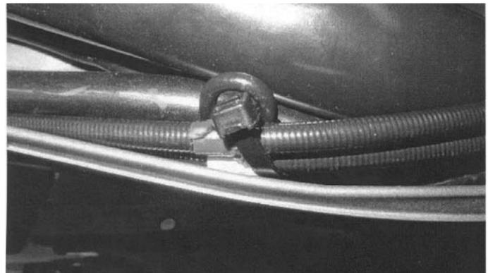
The GREEN marker identifies the throttle opening cable (top), the WHITE marker identifies the throttle closing cable (bottom).
