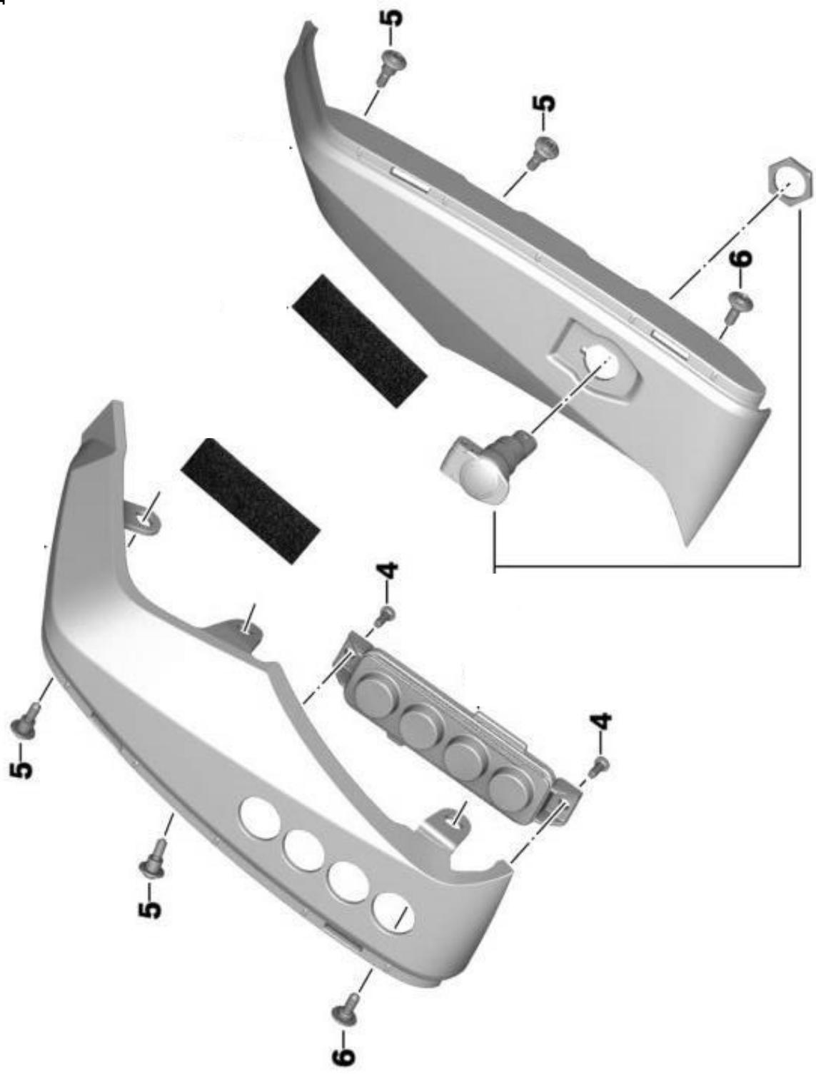
4 = K40x12      5 = Binding Head Screw M5x16-A2-80      6 = M5x14 Without Shoulder
